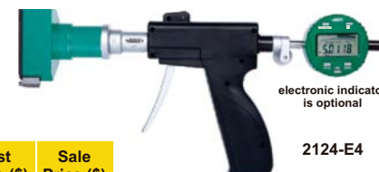
Type C 2-4", carbide measuring points
