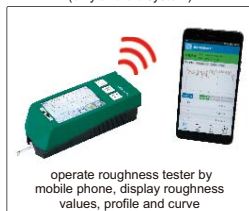
data can be output to Excel by connecting computer via bluetooth or USB cable
